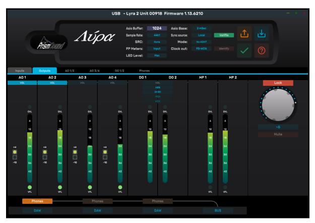
Whilst Lyra can be controlled in a limited way from within the Mac or Windows operating system, or by some audio application programs, most of its detailed features can only be accessed using the Lyra Control Panel app.
