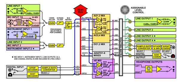
The figure above is a simplified block diagram of the Lyra audio signal paths.
