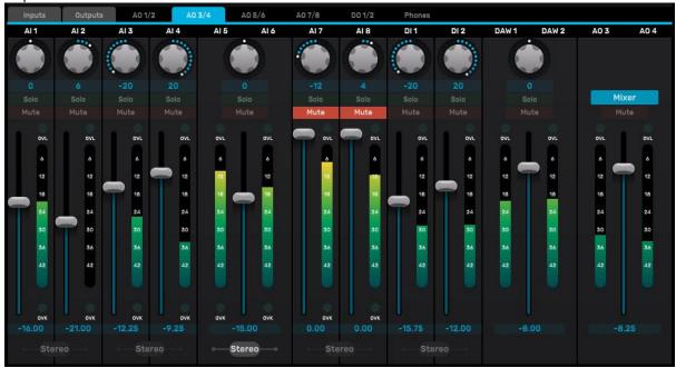
Each input has a fader, a high-resolution <u>peak meter</u>, with overload indication 0.05dB below clipping, plus mute and solo buttons and a pan-pot. By engaging the 'Stereo' button beneath an input pair, the pair is controlled by a single stereo fader, mute button and solo button, and the pan-pots are replaced by a single balance control. The DAW contribution and output strip are always in stereo mode.
